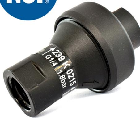
The pre-set EcoReg® fluid regulator is an independent diaphragm pressure regulator that can be installed in all fluid systems. The pressure regulator ensures a constant and precise output pressure independent from the input pressure. The pressure value has been factory preset and cannot be changed. This ensures that no one can manipulate the specified pressure value.
