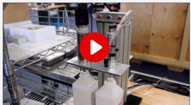
SMAC actuators' repeatable positioning with high speed allows you to more precisely and repeatedly control the dosing amount.
