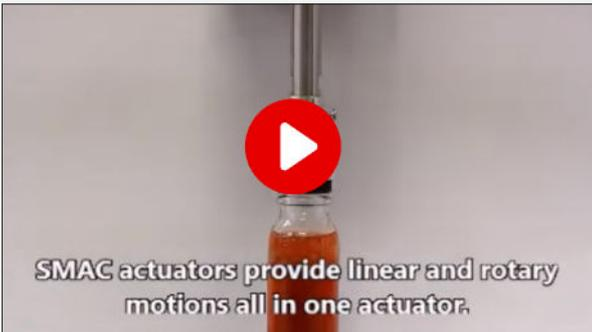
SMAC linear rotary actuator rotates the cap while pushing down. Actuators can press with programmable force and provide torque feedback that informs when the cap has torqued out (or not) to ensure a quality operation.
