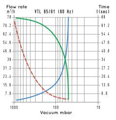
To calculate the emptying time of a volume of  $V_1$ , use the following formula:  $t_1 = \frac{t \times V_1}{100}$
