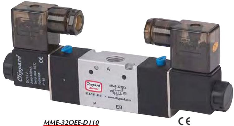
Maximatic® 3-way electronic valves are either N.C. single solenoid spring return or double solenoid spool valves in #10-32 to 1/2" NPT port sizes.
