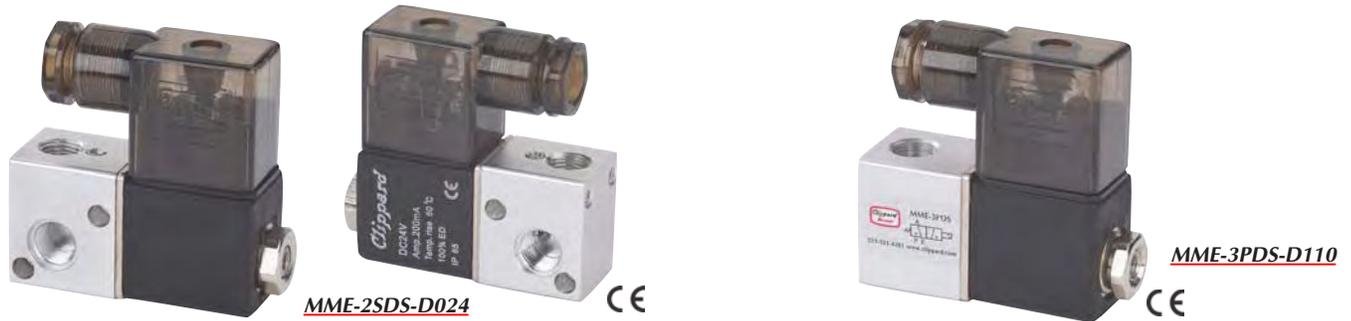
Maximatic® Direct-Acting Valves are single solenoid spring return poppet type valves available as either 2-way or 3-way configurations in ports sizes 1/8" NPT and 1/4" NPT. Hardware to stack multiple valves included with each stacking valve (MME-3SDS and MME-2SDS).
