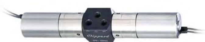
These compact Fill & Bleed circuits are a combination of electronic valves and manifolds used to inflate and vent or release pressure in a controlled system. These circuits are primarily used in applications where a particular pressure, firmness, or position can be controlled with the addition or venting of pressure.
