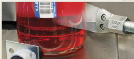
A stainless steel 1" Flat Super Air Nozzle removes condensation from a label prior to scanning.
