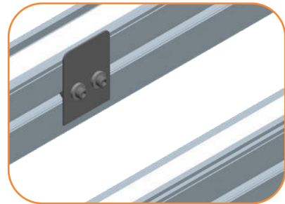
RECOMMENDED ACCESSORY: Pallet Guide Plate minimizes pallet twist
