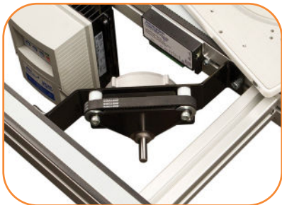
Mini Conveyor Drives Pallet around Corner
