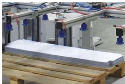
A series of bellows cups lift one plastic part at a time off of a pallet.
