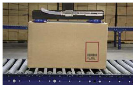
Compressed air use is minimized by selecting the exact vacuum level required to lift the heavy, porous cardboard cartons.
