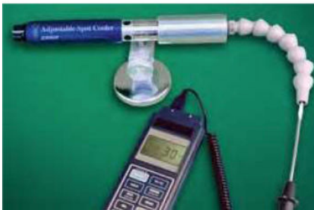
The Model 3825 Adjustable Spot Cooler can produce temperatures from -30° to +70°F (-34° to +21°C).
