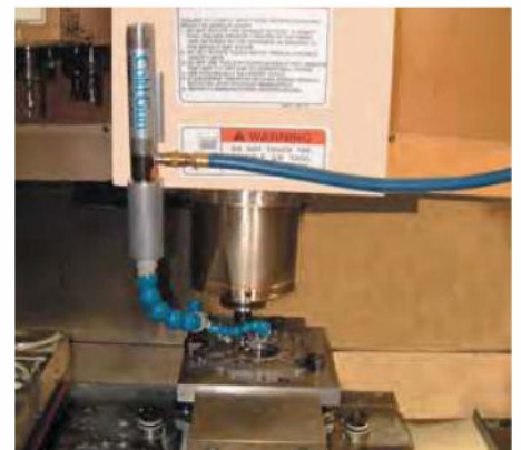
The Model 5315 Cold Gun cools a two flute 3/8" carbide cutter on a CNC, increasing tool life by 50%.
