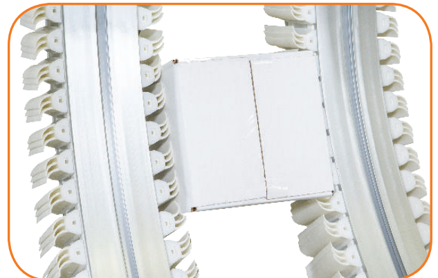
Products are wedged between opposing conveyors
