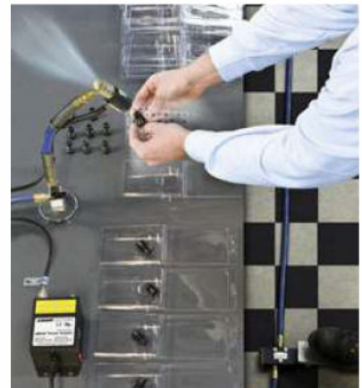
The Gen4 Model 8910 Instant Static Elimination Station removes contaminants on plastic fittings prior to packaging.
