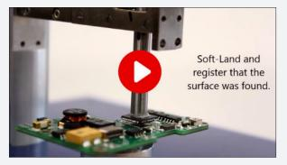
The precision Z-theta motion within one small actuator, providing a convenient pick, orient and place. The unique Soft-Land function allows the unit to gently land on a delicate component with a controlled force, avoiding damage to the component.
