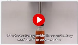
SMAC linear rotary actuator rotates the cap while pushing down. Actuators can press with programmable force and provide torque feedback that informs when the cap has torqued out (or not) to ensure a quality operation.
