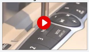
In-line durability test. Measuring click point, force and displacement. Report force vs. position with SPC data collection. Life testing of components as well as measurement and QA reporting functions in one unit.
