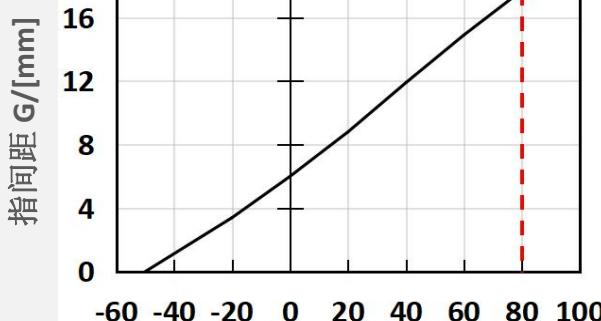
\*Working pressure P[kPa] (safe limit +80kPa)
