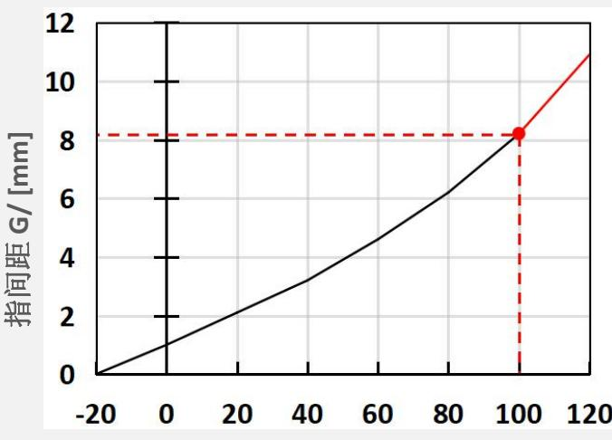
\* Working pressure P[kPa] (safe limit +100kPa)
