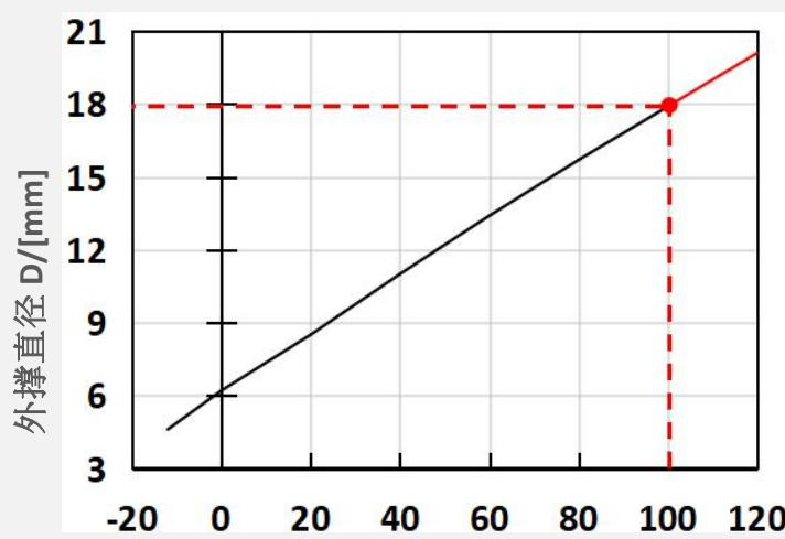
\*Working Pressure P [kPa] (Safe limit+100kPa)
