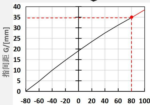
\*Working Pressure P[kPa](Safe limit+80kPa)
