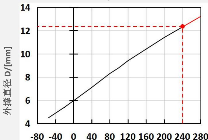
\*Working Pressure P[kPa] (Safe limit+240kPa)
