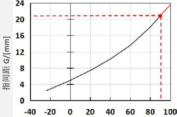
\*Working pressure P [kPa] (safe limit +90kPa)
