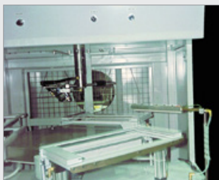
Standard ion luftkniv renser metalrammer inden pulverlakering.
