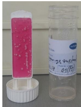
Coolant after three days: No thermal disinfection bacteria 10^4 cfu/ml fungi 10^4 cfu/ml (cfu = colony-forming units)
